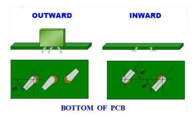
2.5mm Span Standard Configuration
